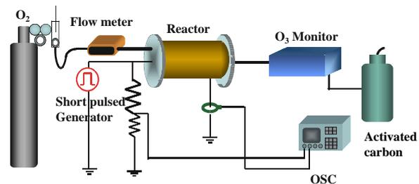
Figure 6. Experimental set-up for production of ozone
