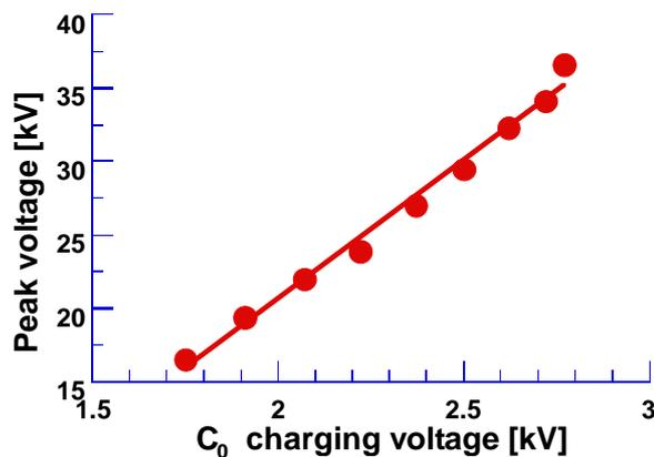
Figure 2. Peak voltage of MPC as a function of the charging voltage to C<sub>0</sub>.
