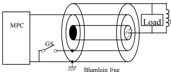
Figure 3. Schematic diagram of the short-pulsed generator.
